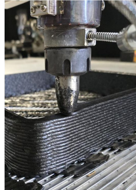
Large-scale additive manufacturing of the composite mould (left) and tape shearing with the iCOMAT RTS process (right)
