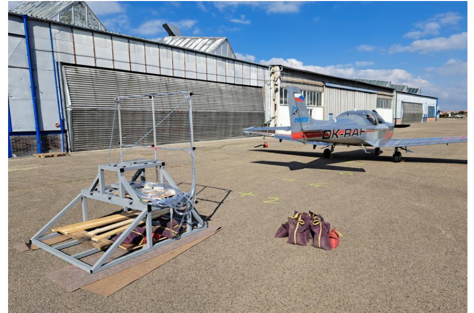
Open-air acoustic test set-up with the demonstrator platform
